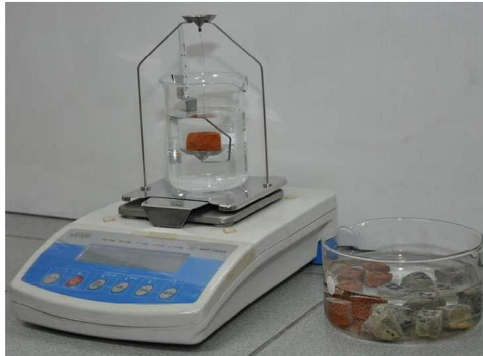
Fig. 1. The set for marking of volume density of stone materials
