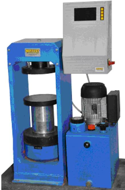
Fig. 3. Hydraulic press for testing compressive strength
