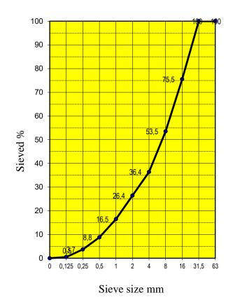
Rys. 1. Aggregate grading curve for this example
