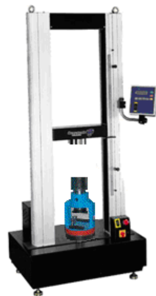
Rys. 6.2. Universal flexural testing machine.
